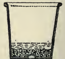
FIG. 26.—Section of Pot showing Crocking.
